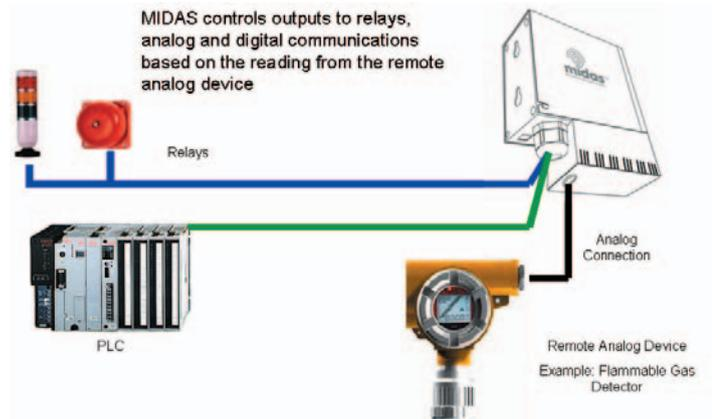
Any MIDAS® detector can be fitted with the optional analog input module that accepts the analog signal from a remote device. MIDAS® can then be configured to display the remote system's analog reading on the local LCD, trigger relays and provide a digital output via Modbus/TCP Ethernet.
