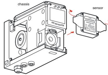
Diagram 24. Fitting/replacing sensor cartridge
