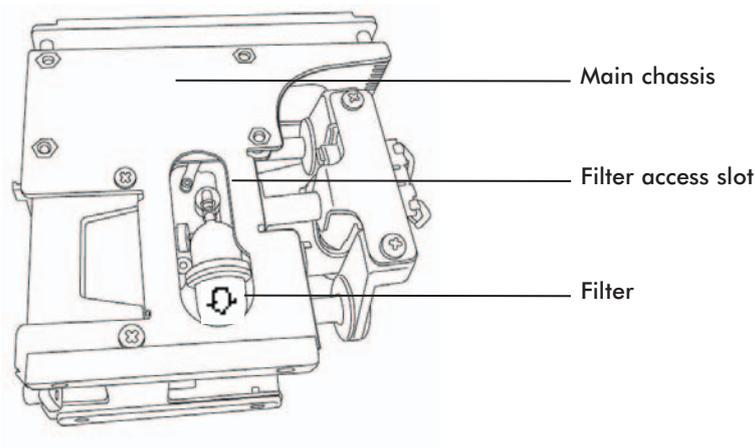
7. Carefully disconnect both sides of the filter from the pump manifold.
