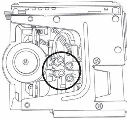
8. Slide the pump module out and disconnect the connector from the pcb.
