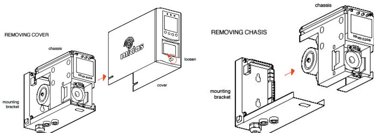
Diagram 8. Mechanical installation
