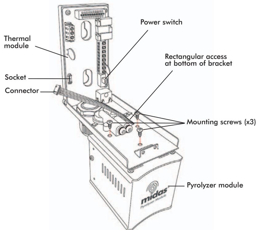
8. Offer the pyrolyzer module up underneath the mounting bracket ensuring that the fitting at the top rear of the pyrolyzer mates with the sample inlet port at the bottom of the mounting bracket.
