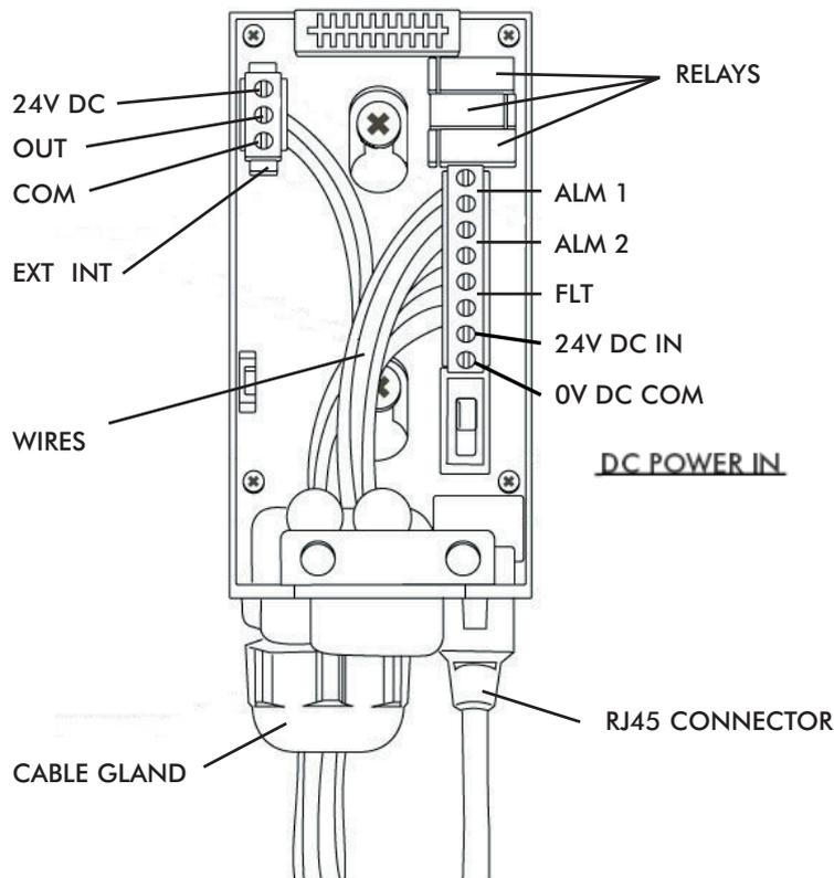
The terminals used are suitable for conductors of 24 to 14 AWG (0.5 to 1.8mm Dia.). The use of 16 AWG (1.5 mm Dia.) conductors is recommended.
