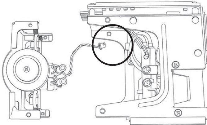
9. Fit the new pump module following the steps above in reverse order.
