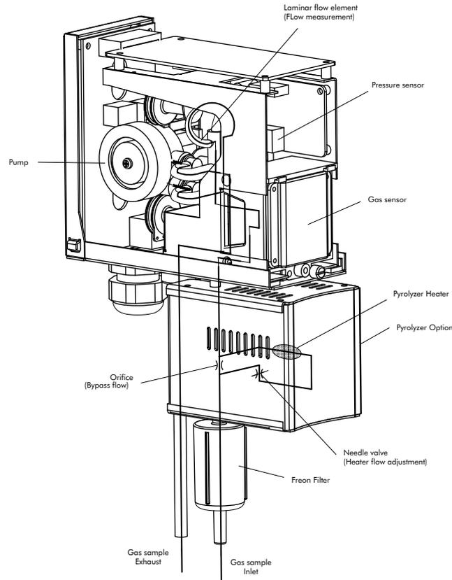
Diagram 37 shows in diagrammatic form how the gas sample flows through the various components. It shows how the instrument controls, monitors and measures the gas sample flow and signals any fault conditions to the user via the LCD screen, e.g. due to flow problems caused by pump failure, or failure of the pyrolyzer unit, etc.
