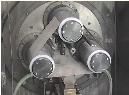
A diamond electroplated wire slices a sapphire ingot.
