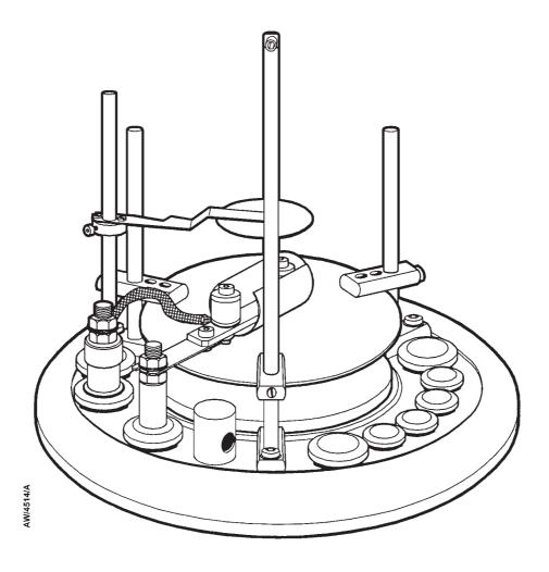
Figure 1 - Source Shutter mounted on the AUTO 306 baseplate
