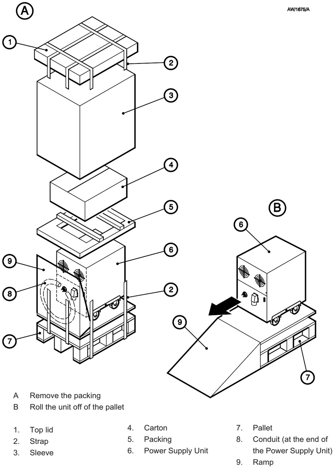
Figure 13 - Unpack the EB3 3 kW Power Supply
