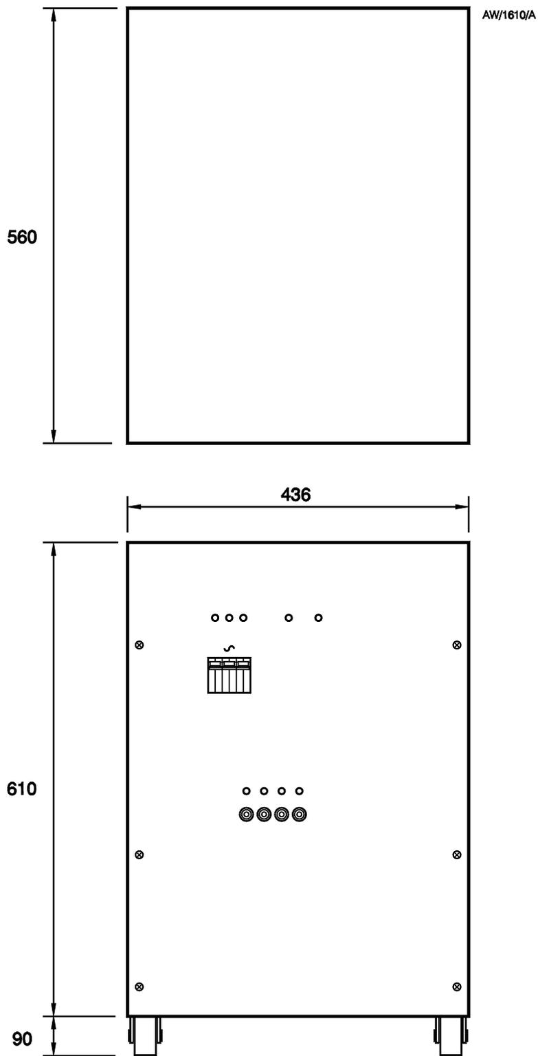
Figure 10 - Dimensions of the EB3 Power Supply Unit (mm)
