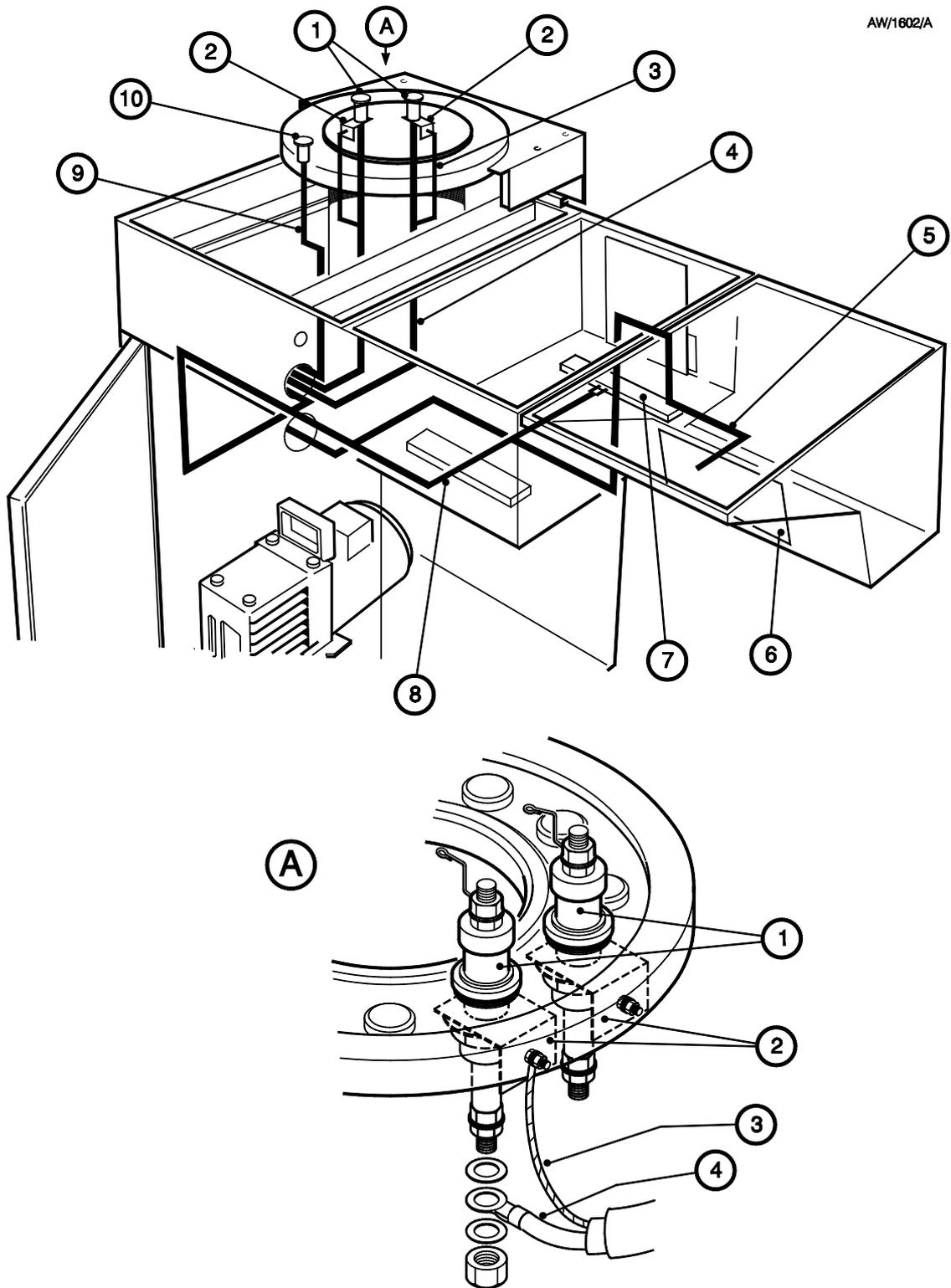
Figure 29 - Cable routes for the Power Supply Unit electrical connections
