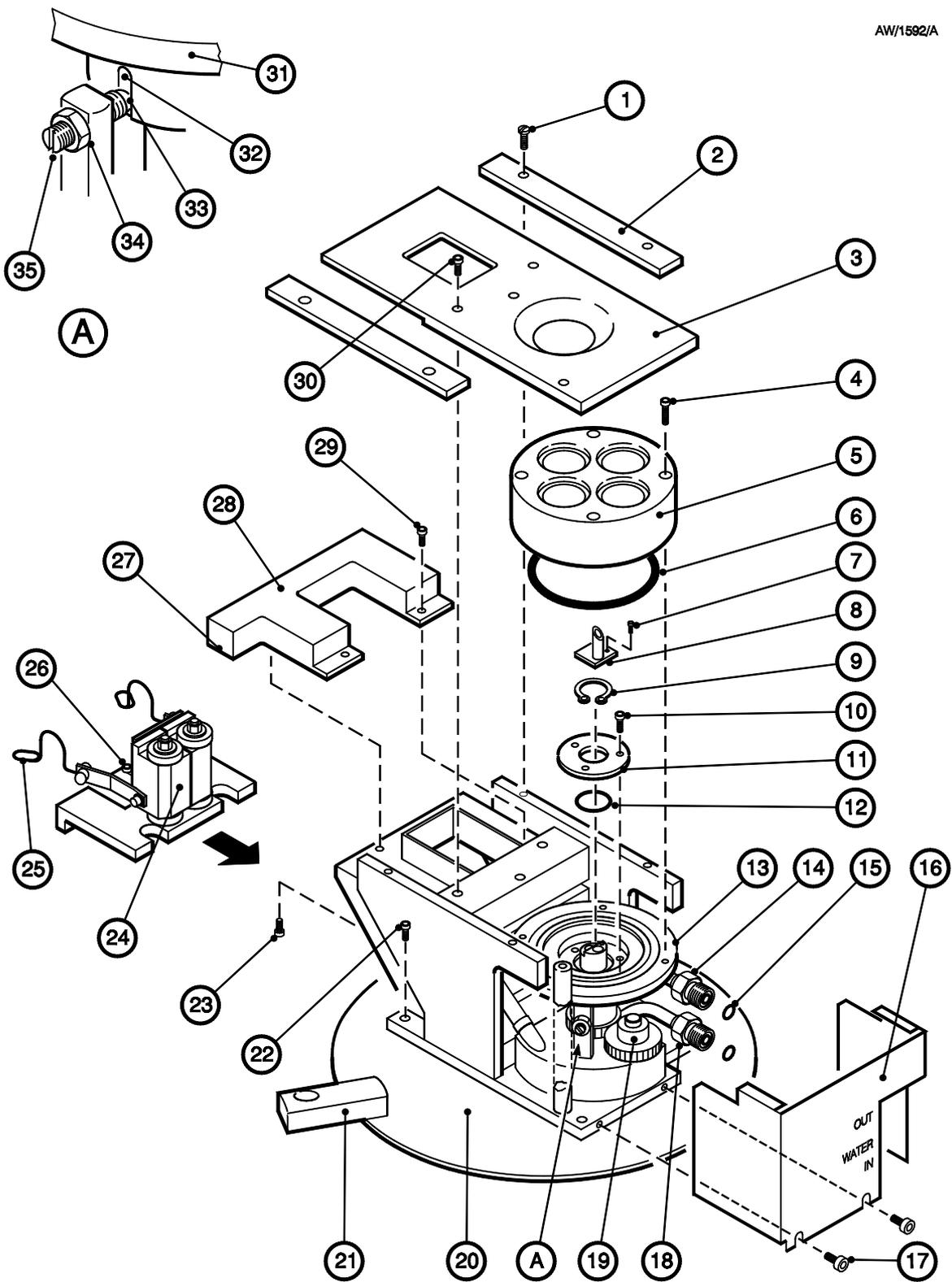
Figure 20 - Components of the EB3 Multihearth Electron Beam Source
