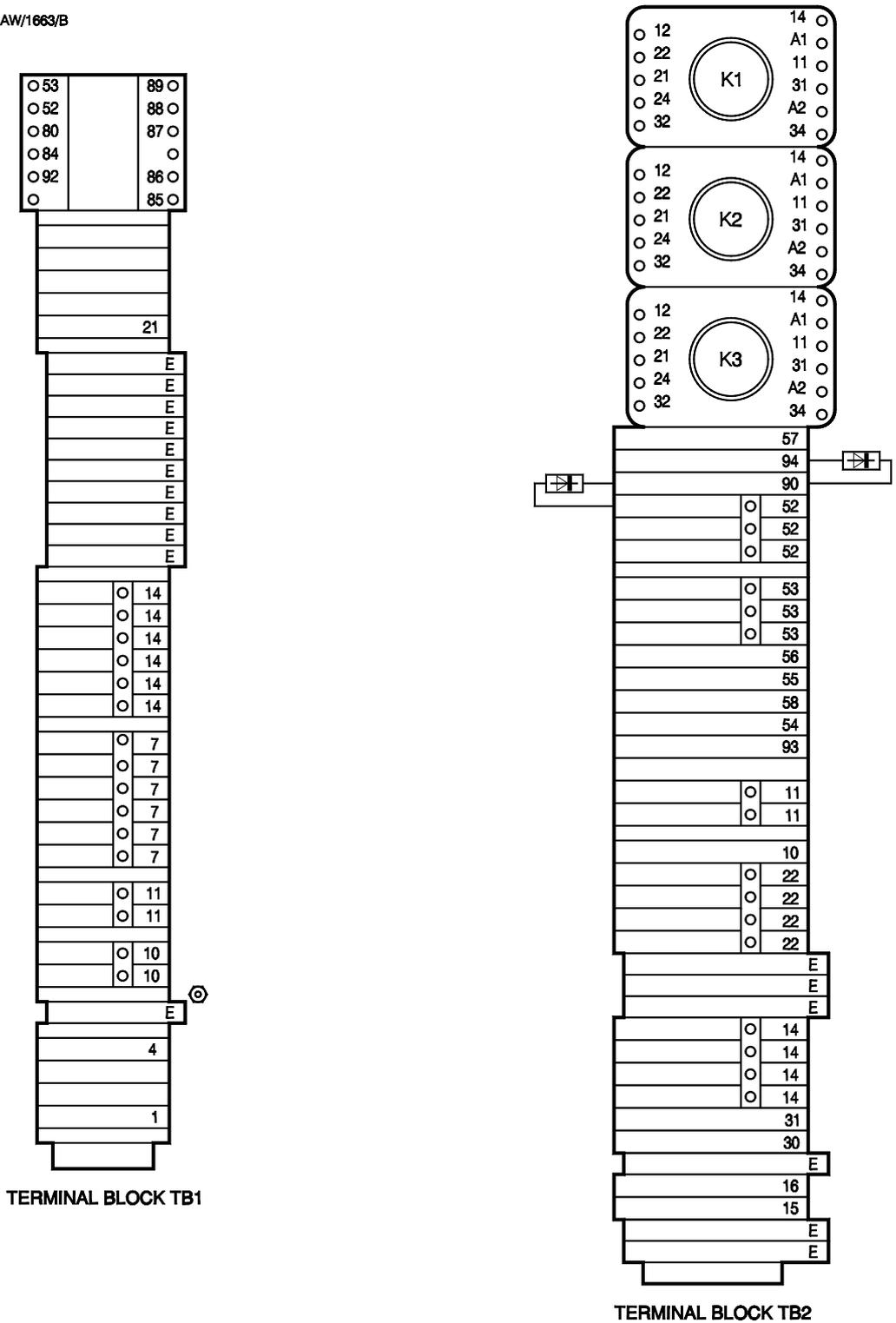
Figure 31 - Configuration of the terminal blocks
