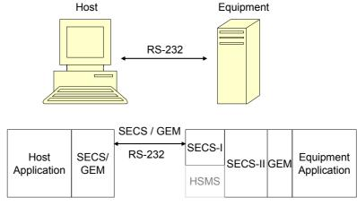
FIGURE 11-2: SYSTEM CONFIGURATION USING RS-232
