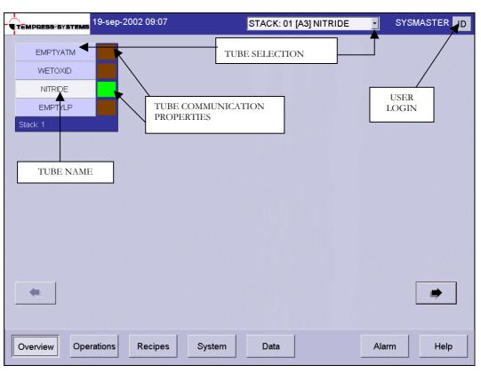
FIGURE 4-2: TUBE SELECTION AND PROPERTIES
