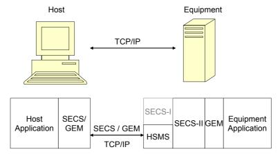
FIGURE 11-3: SYSTEM CONFIGURATION USING TCP/IP
