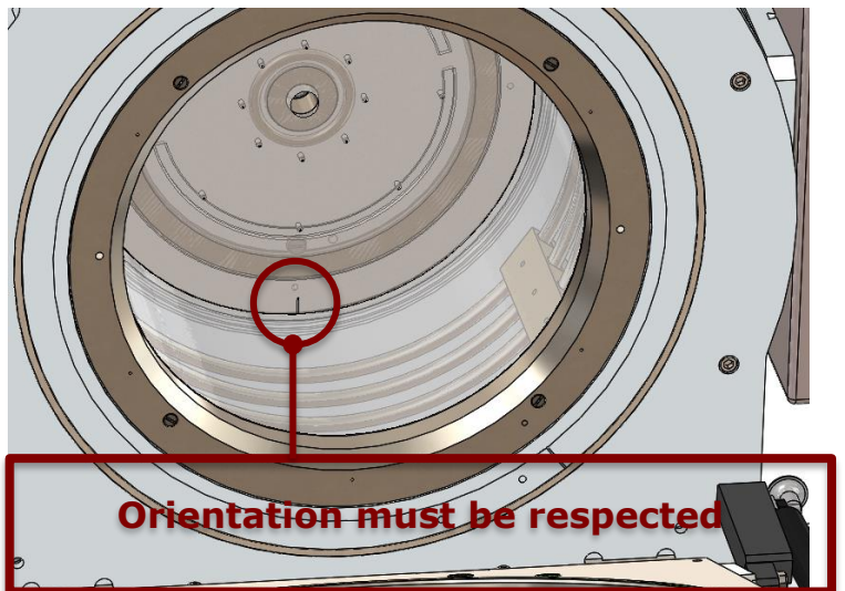
Figure 13 Detailed view of the reactor ICP with the shower gas and alignment mark
