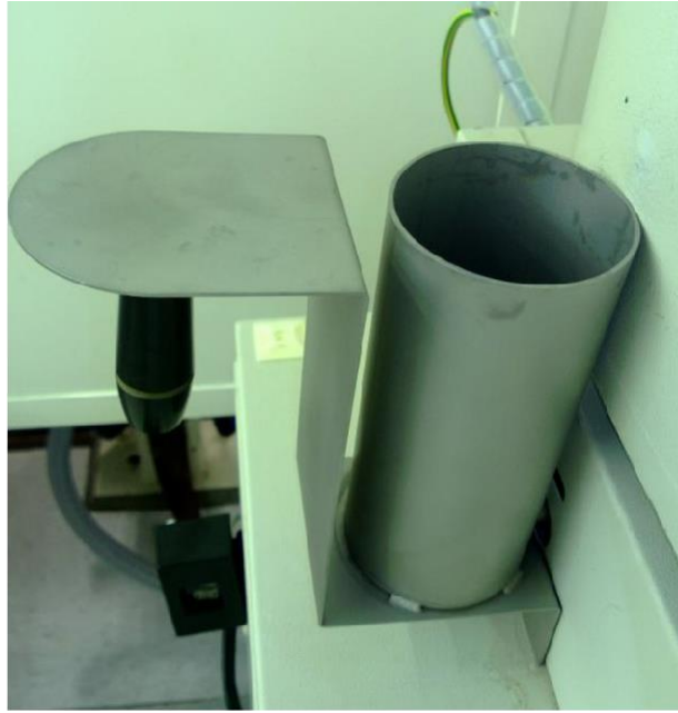
Figure 3 – Liquid Nitrogen fill funnel on the side of the chamber
