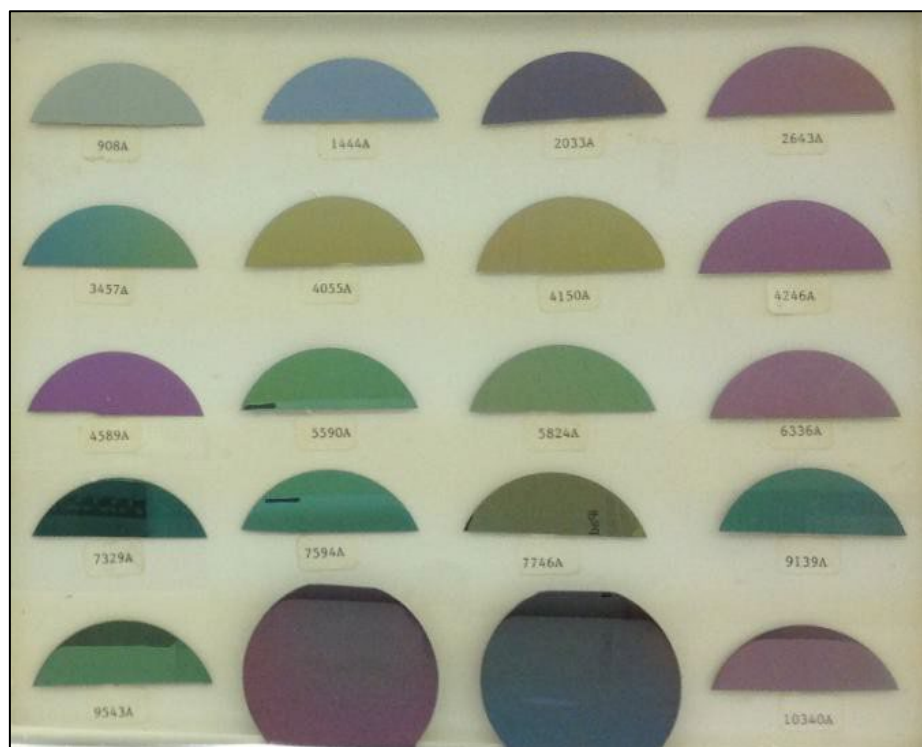
Figure 10 – Wafer Oxide Thickness Color Guide
