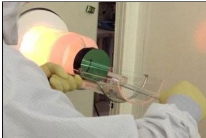
Figure 6 – Quartz boat being loaded/unloaded using the short quartz rod and glass boat loader/unloader.
