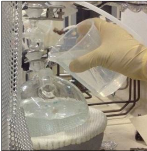
Figure 3 – Filling DI Water Bubbler for Wet Oxidation
