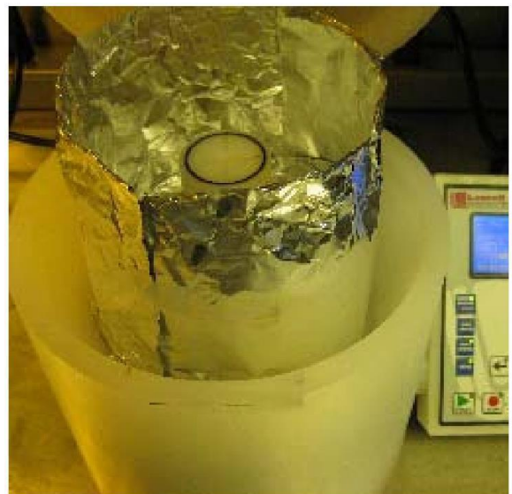
Figure 2 Aluminum foil cylinder lining spin coater bowl
