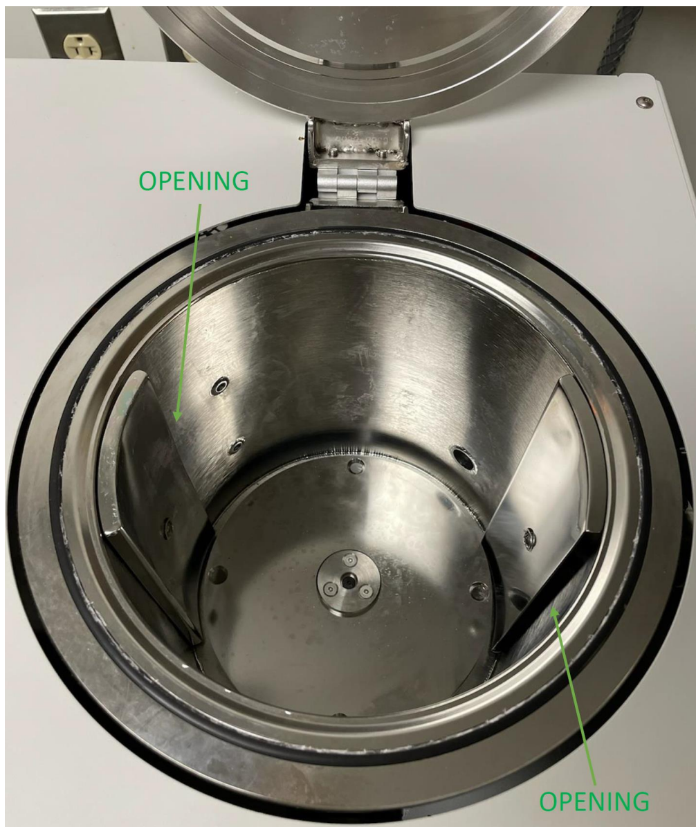
Fig. 2. Baffle Opening Orientation: The orientation recommended by the vendor is shown above. The baffle orientation influences residence time and likely deposition rate and uniformity.
